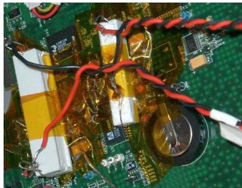
Figure A2.2 Power resistors are applied to a suspect circuit
